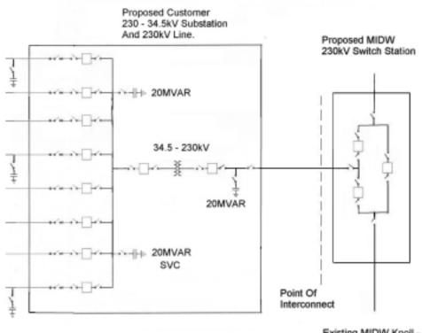
34.5kV Switched Capacitor Banks No Greater Than 20MVAR Each Existing MIDW Knoll -WERE Summit 230kV Line
